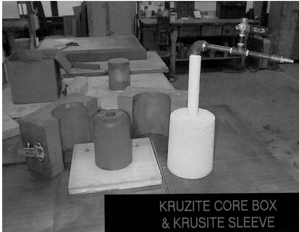
Figure 15 Pressure cap made from Kruzite castable ceramic with fused silica (Fusil) pressurization tube and gas line fittings with T-valve argon gas line
