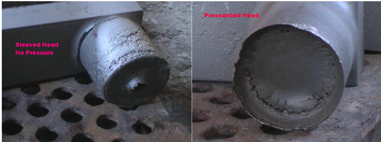
Figure 29 Non-pressurized riser from plate T3-3X cast using exothermic sleeve (above left) and top of pressurized riser from plate T3-4X (above right)
