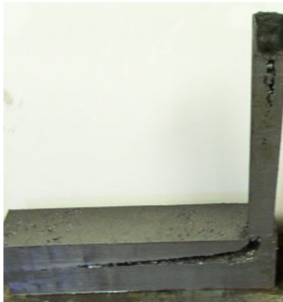
Figure 20 Section taken through plate T1-3X at the vent end shows the interior hole created by the argon leak
