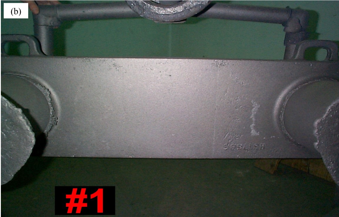
Figure A4. (a) Schematic of the revised rigging design, and (b) a picture of the clean cope surface resulting from this rigging.
