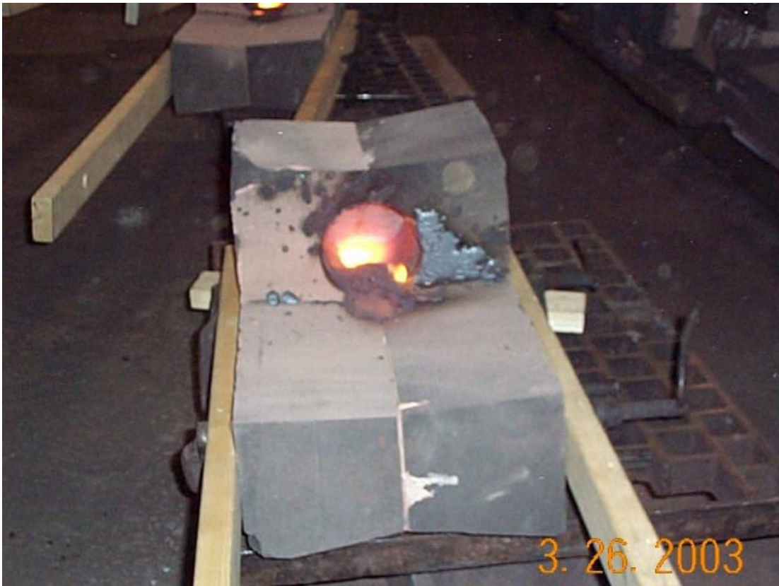
Figure 9 A tilting mold after pouring and tilting.
