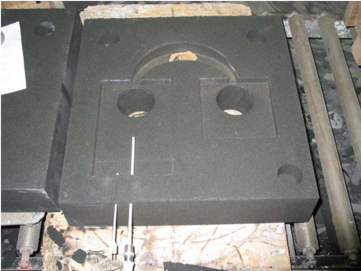
Figure 9 Mold cope, with two thermocouples inserted.
