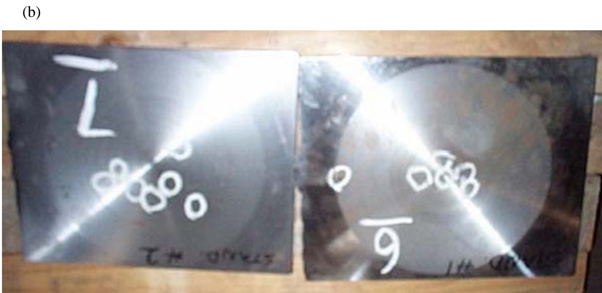
Figure 9. Comparison between simulation and experimental results: (a) Top view of final simulated inclusion locations. Inclusions shown at 3x magnification; (b) photo showing inclusion locations on the cope surface of two experimental plates.
