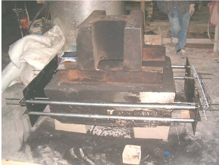
Figure 5. Flask assembled around the T-section casting mold.
