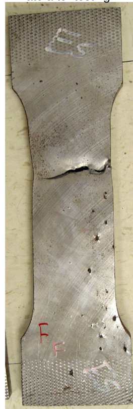
Figure 35 From left to right, radiograph used to determine porosity in plate E5, plate E5 after testing, and plate E5 simulation Von Mises stress at failure.
