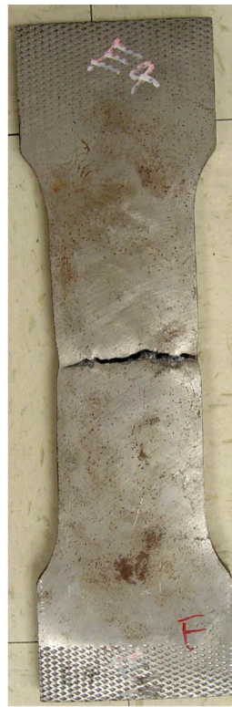
Figure 34 Radiograph used to determine porosity in plate E4, E4 after testing, and E4 simulation at failure.
