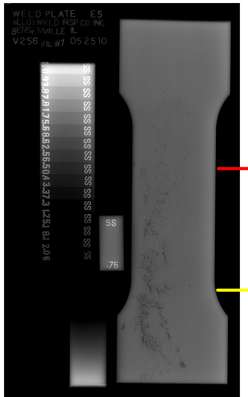
Figure 35 From left to right, radiograph used to determine porosity in plate E5, plate E5 after testing, and plate E5 simulation Von Mises stress at failure.
