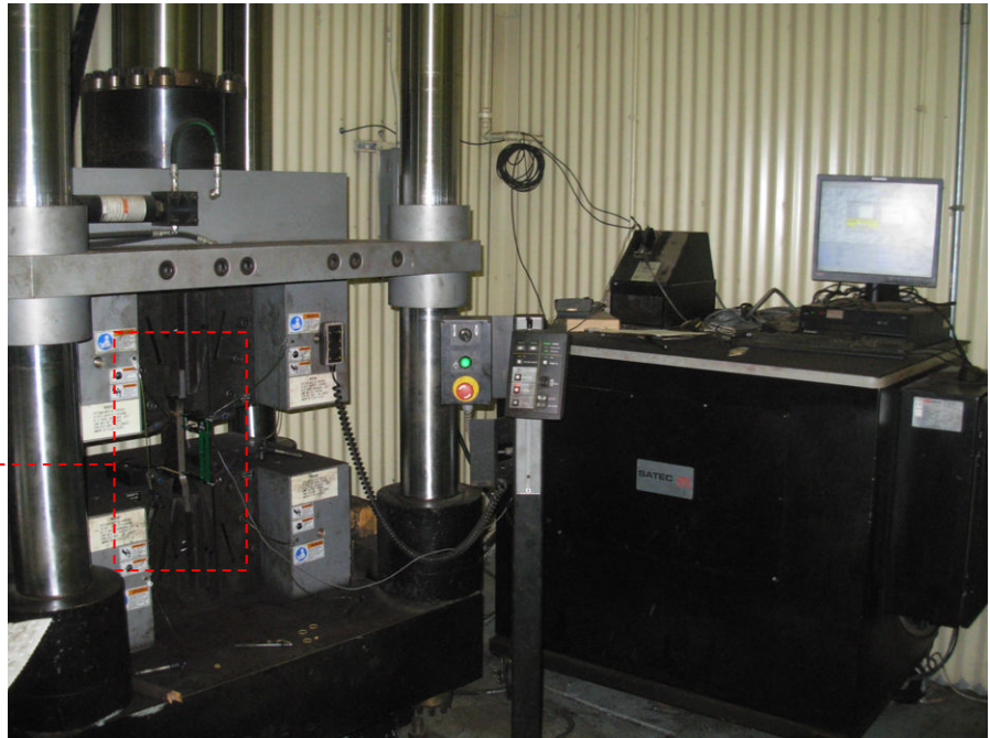
Figure 8 View of test coupon with 6" extensometer fixed to narrow face (image at left) and test machine and controller (image at right).
