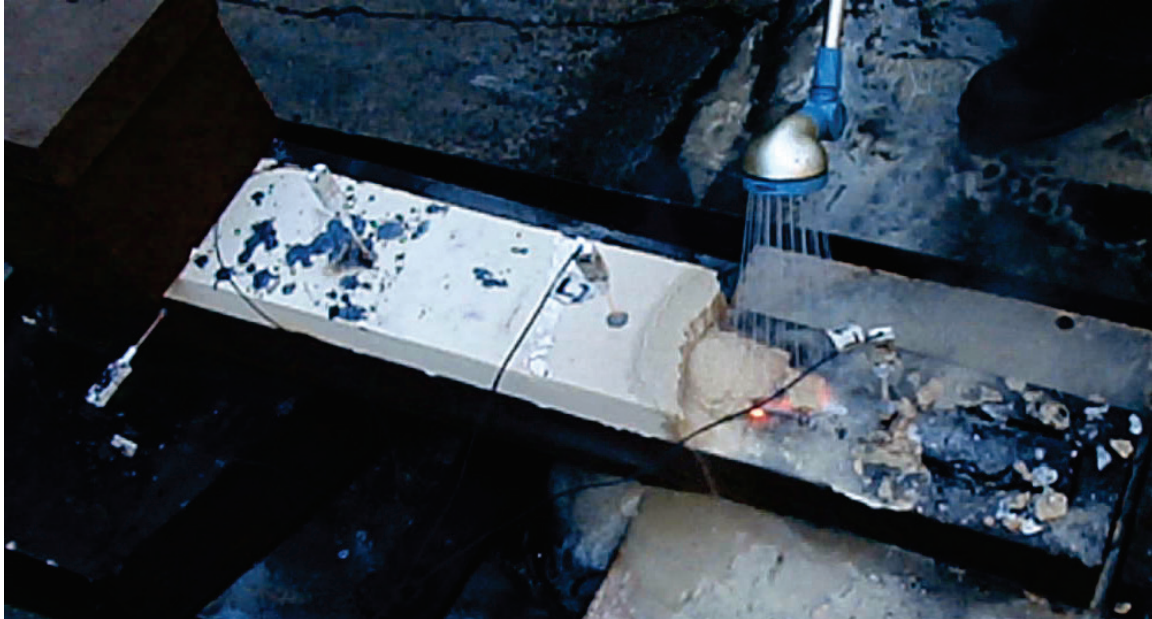
Figure 1. Modified ablation casting of a long bar, where only the cope is water-soluble.
