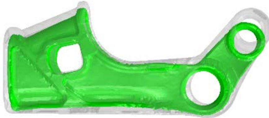
Figure 5. Deformed shape at room temperature as predicted by the finite element simulation.
