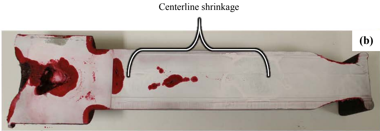
Figure 12 Dye penetrant test results from the (a) CGPS casting and (b) the second gravity-poured casting.
