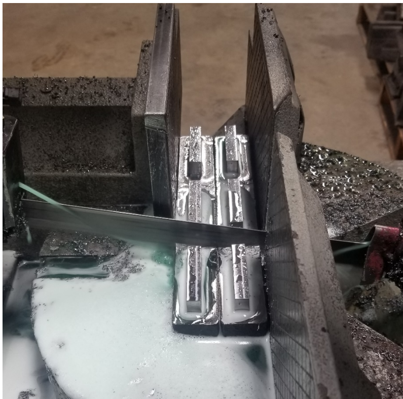
Figure 9 Shows two Charpy leg after it has gone through its first machining operation. Each leg is being cut into three pieces before the final machining operation.
