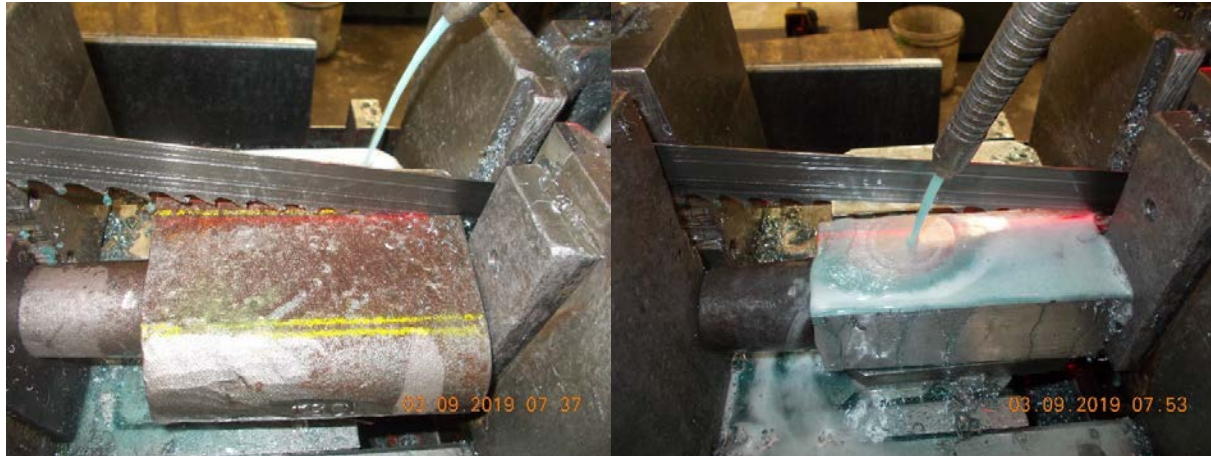
Figure 10 Shows an E.R. Charpy bar being cut down to shape before it goes to the mill.
