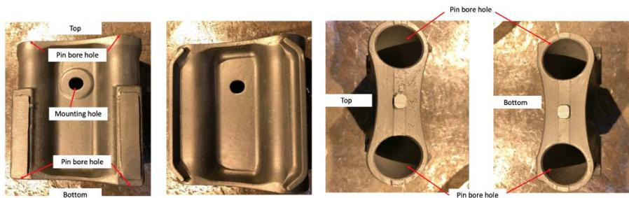
Figure 1. As-cast high aluminum manganese steel shoe.
