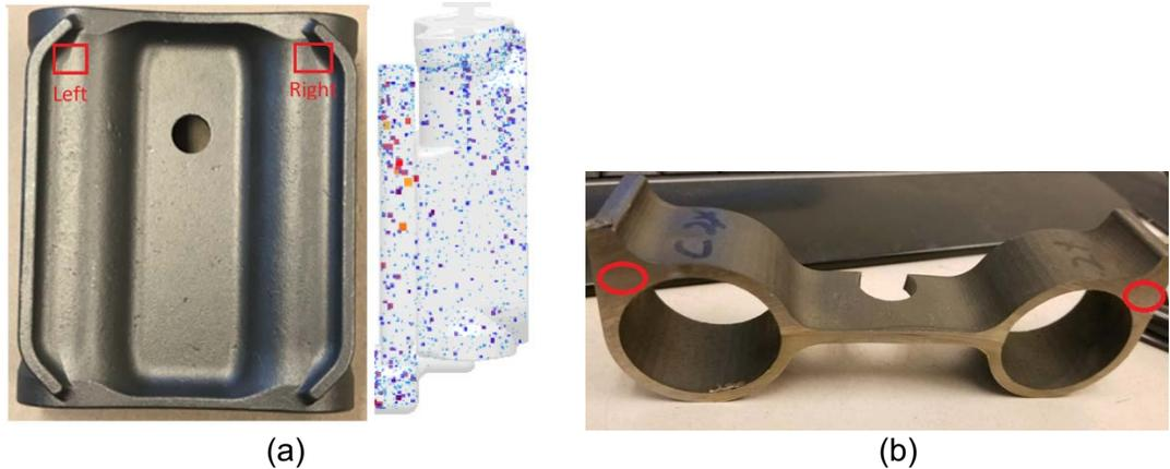
Figure 20 (a) The castings were sectioned for inclusion analysis in the two areas (left and right) denoted by the highlighted regions. These areas were shown by inclusion modeling to have the highest concentration of inclusions. (b) Sectioning plane showing the exact location of the inclusion analysis highlighted in red.
