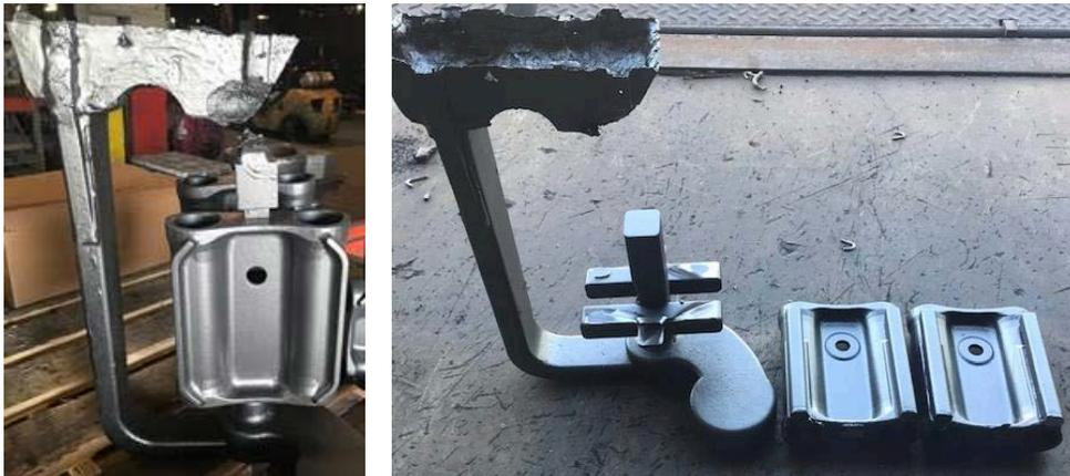
Figure 9. Naturally pressurized (NP) with side sprue
