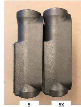
Figure 15. Castings after heat treatment for traditional investment gating system #5
