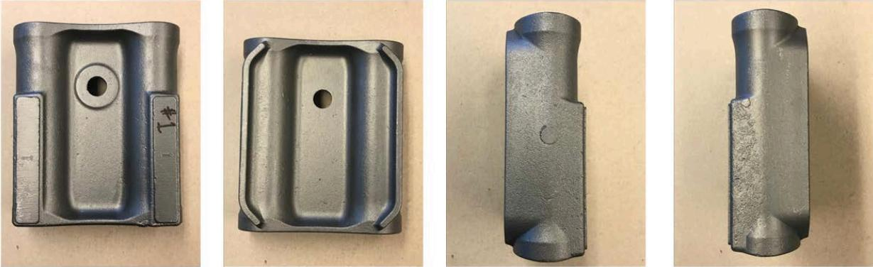
Figure 11. Casting after heat treatment for traditional investment gating system #1
