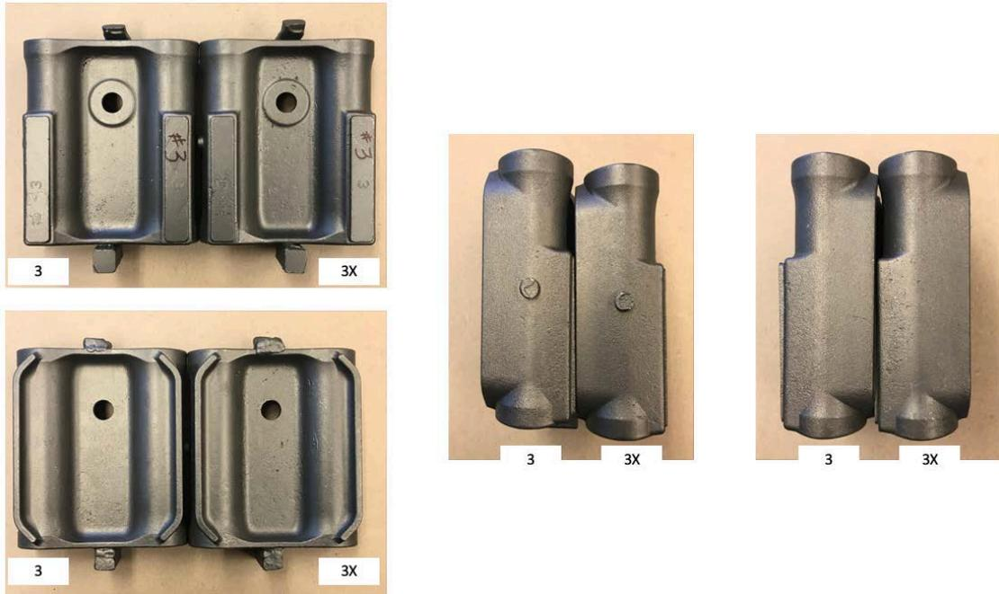
Figure 13. Castings after heat treatment for traditional investment gating system #3
