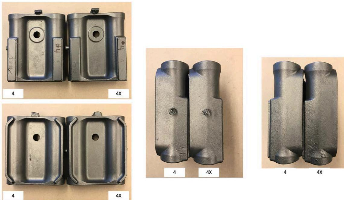
Figure 14. Castings after heat treatment for traditional investment gating system #4
