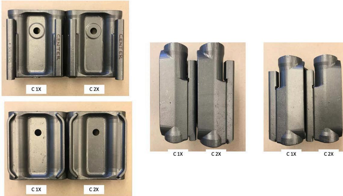
**Figure 17. Castings after heat treatment for naturally pressurized with center sprue**
