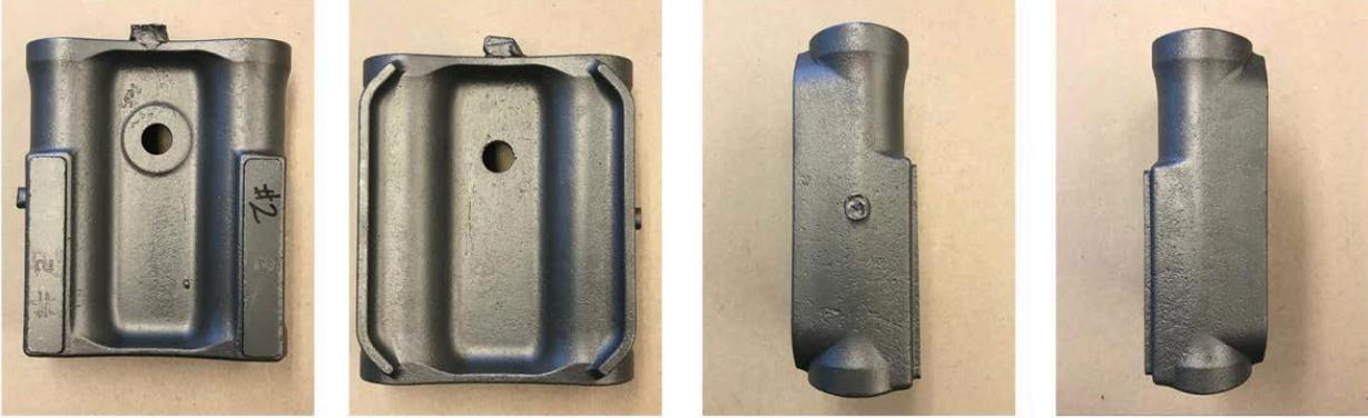
Figure 12. Casting after heat treatment for traditional investment gating system #2
