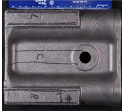
Figure 19. Tensile specimen locations in each shoe
