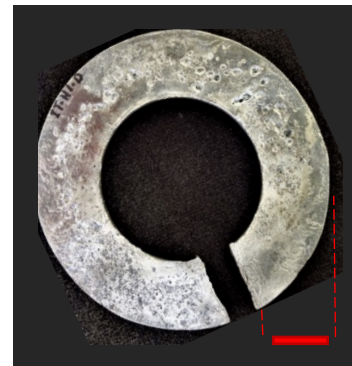
Cope surface Media blasted
