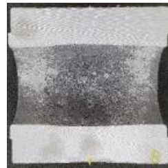
Core surface "as cast"
