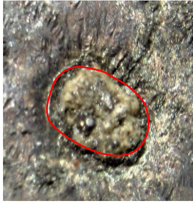
(a) Inclusion example, as cast
