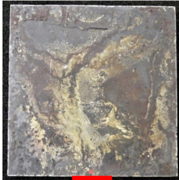
Inclusions Hand Marked on Cope Surface
