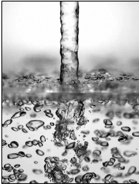
Figure 1. Air bubbles near a plunging liquid water jet by 'Jesse Belden (NUWC) and Tadd T. Truscott (BYU)' [1].
