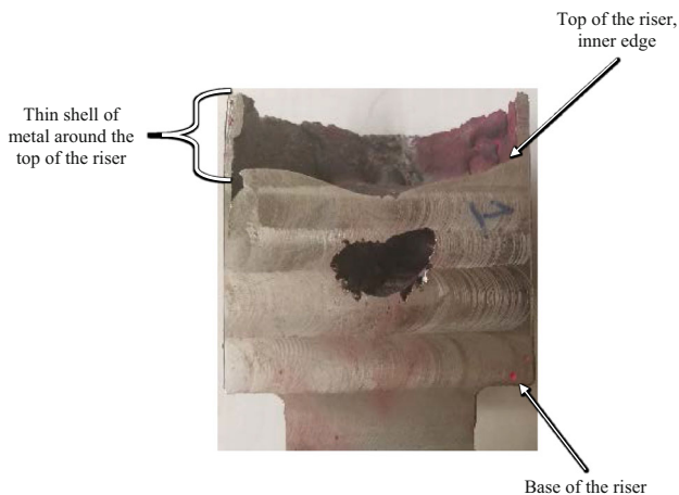
Figure 11. Photograph of the sectioned riser from the CGPS casting.
