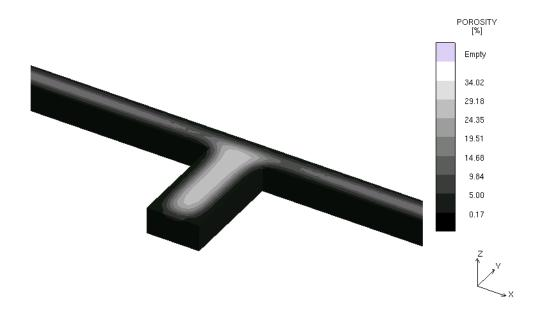
Figure 3: Predicted distribution of porosity,  $f_p^l$ , neglecting solid deformation.
