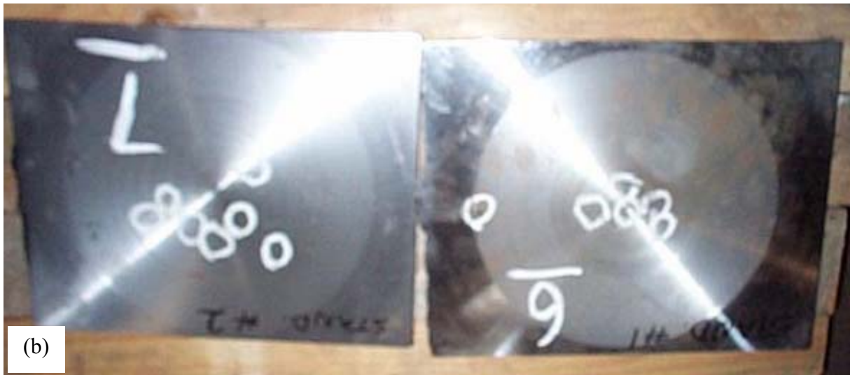
Figure 3: Comparison between simulation and experimental results: (a) Top view of final simulated inclusion locations. Inclusions shown at 3x magnification; (b) photo showing inclusion locations on the cope surface of two experimental plates.
