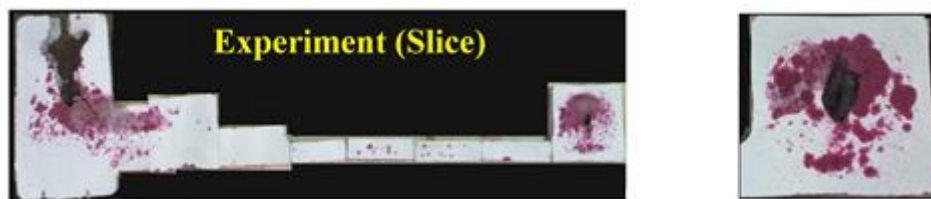
Figure 4. Porosity distribution observed in the Mn-steel casting: vertical slices through the casting at mid-width, with the red areas showing microporosity that is visualized using dye penetration testing.
