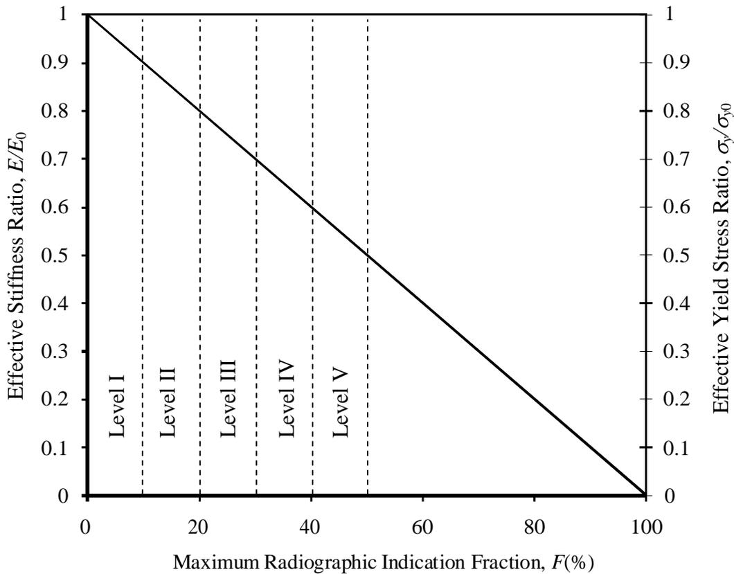
**Fig. 3. Relationship between effective mechanical properties and the maximum radiographic indication fraction,  $F$ . Properties are normalized with their sound values,  $E_0$  and  $\sigma_{y0}$ .**
