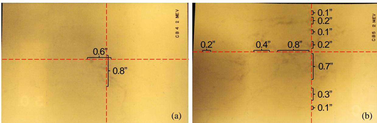
**Fig. 7. Examples of measurements performed on the ASTM E186 reference radiographs to obtain estimates of the maximum indication fraction,  $F$ . (a) CB4:  $F_{horizontal} = 0.6''/4.7'' = 13\%$ ;  $F_{vertical} = 0.8''/3.1'' = 26\%$ . (b) CB5:  $F_{horizontal} = 1.4''/4.7'' = 30\%$ ;  $F_{vertical} = 1.7''/3.1'' = 55\%$ .**
