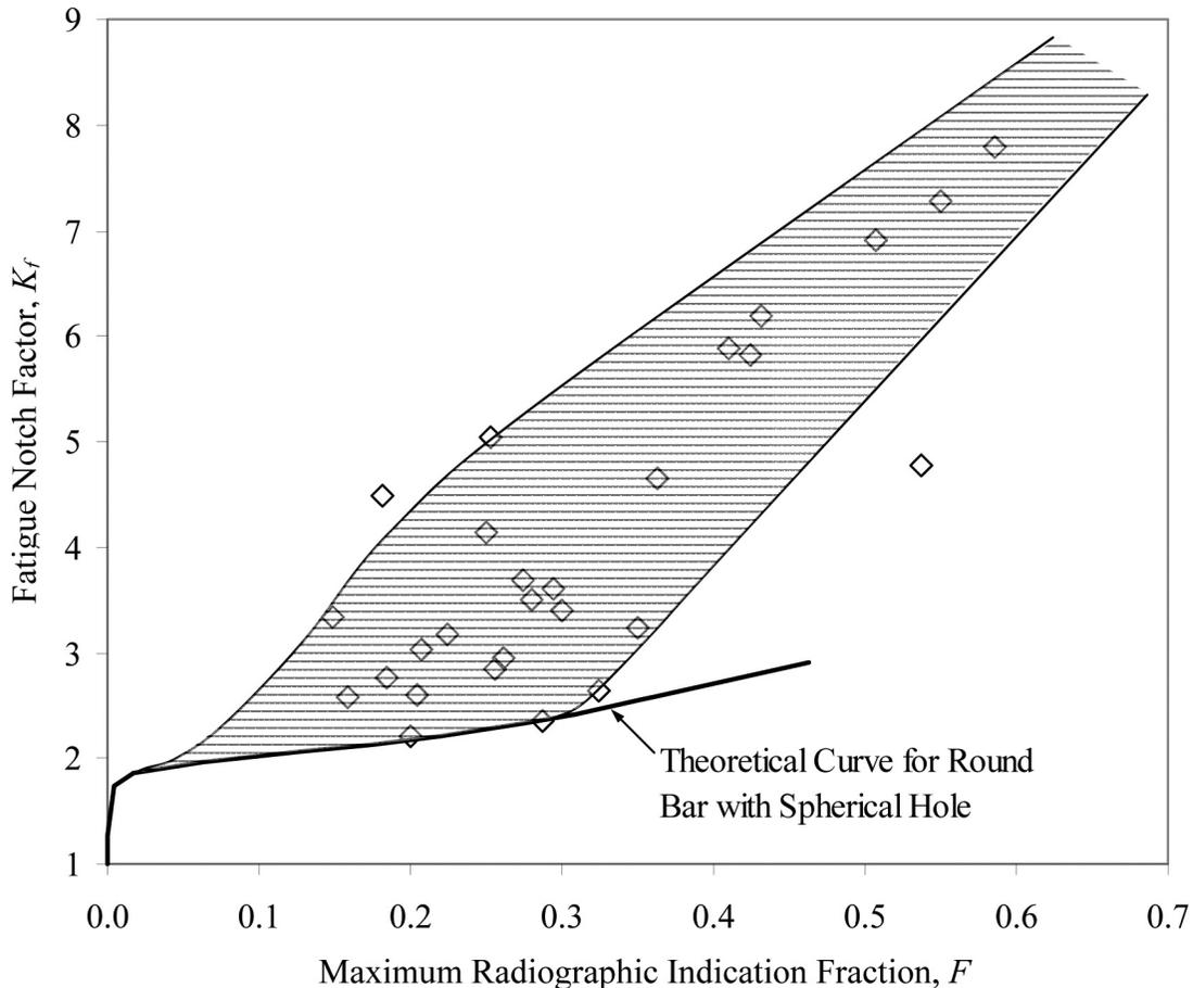
Fig. 6. Fatigue notch factor,  $K_f$ , as a function of the maximum indication fraction,  $F$ .
