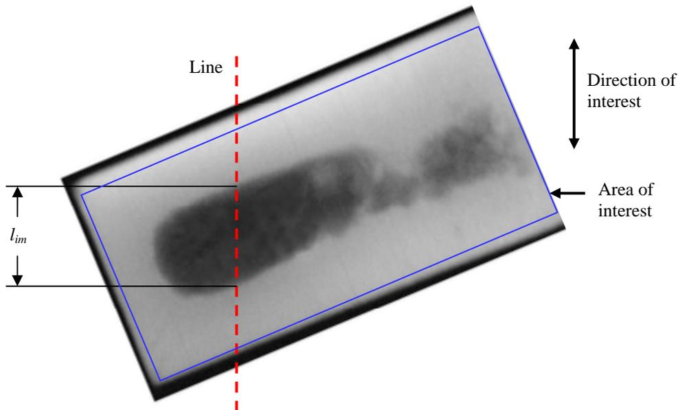
**Fig. 1. Example of the measurement of the maximum total indication length,  $l_{im}$ , on a radiograph.**
