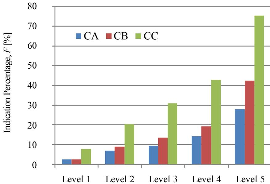
**Fig. 8. Measured maximum indication fraction,  $F$ , as a function of severity level for the shrinkage reference radiographs of ASTM E186.**
