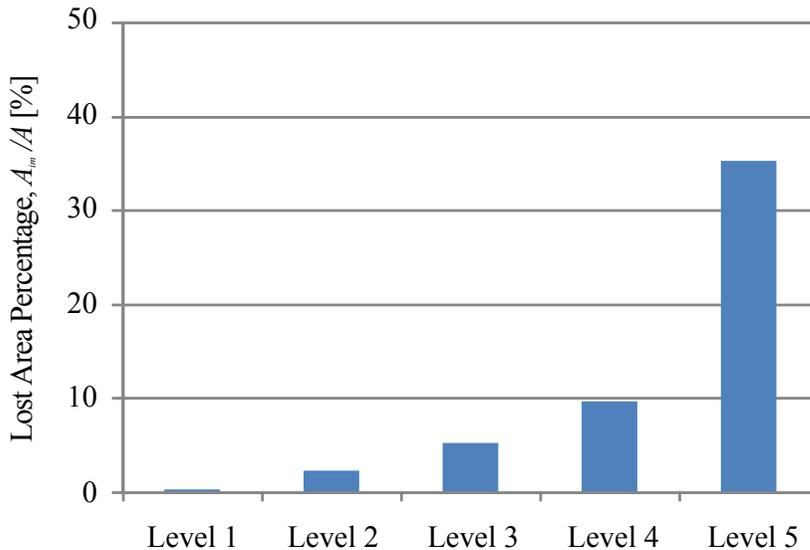
**Figure 9. Lost cross-sectional area percentage as a function of severity level for the shrinkage reference radiographs of ASTM E186; the voids corresponding to the indications on the radiographs are assumed to have a square cross section inside of a 3" by 3" square bar.**
