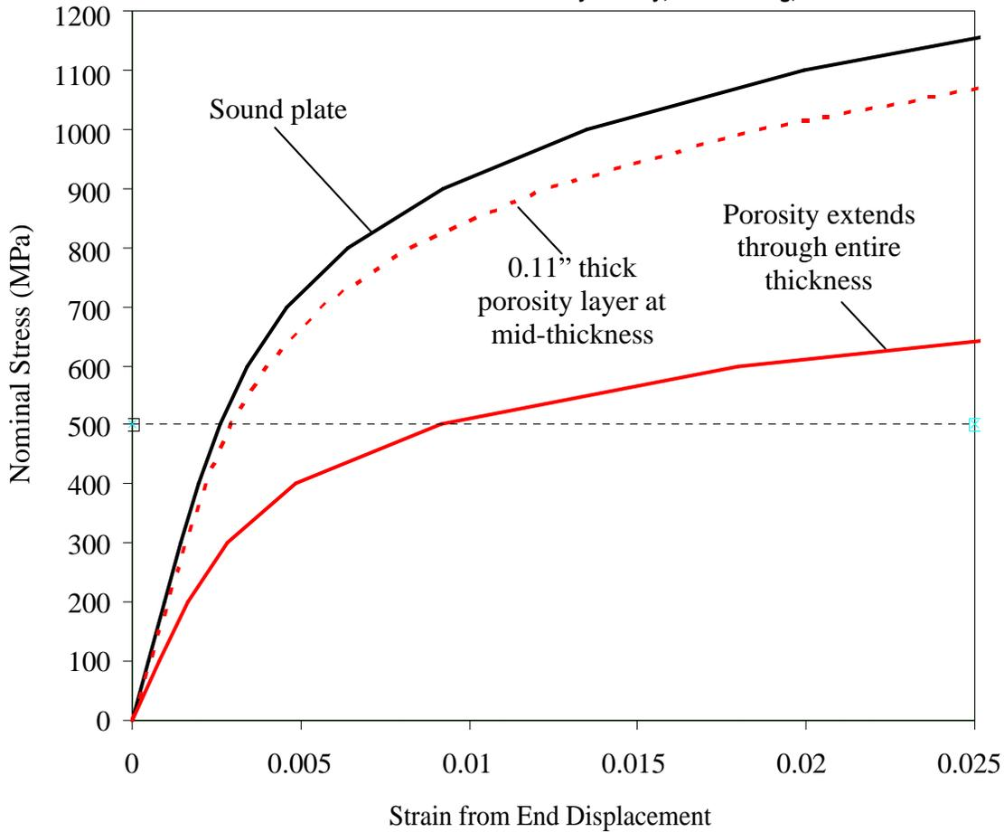
**Fig. 5. Predicted stress-strain curves for the 1" thick plate of Figure 4. The three curves correspond to the porosity distributions shown in Figures 4(a), 4(c) and 4(e). The horizontal dashed line indicates the load of 500 MPa applied in the stress results shown in Figure 4.**
