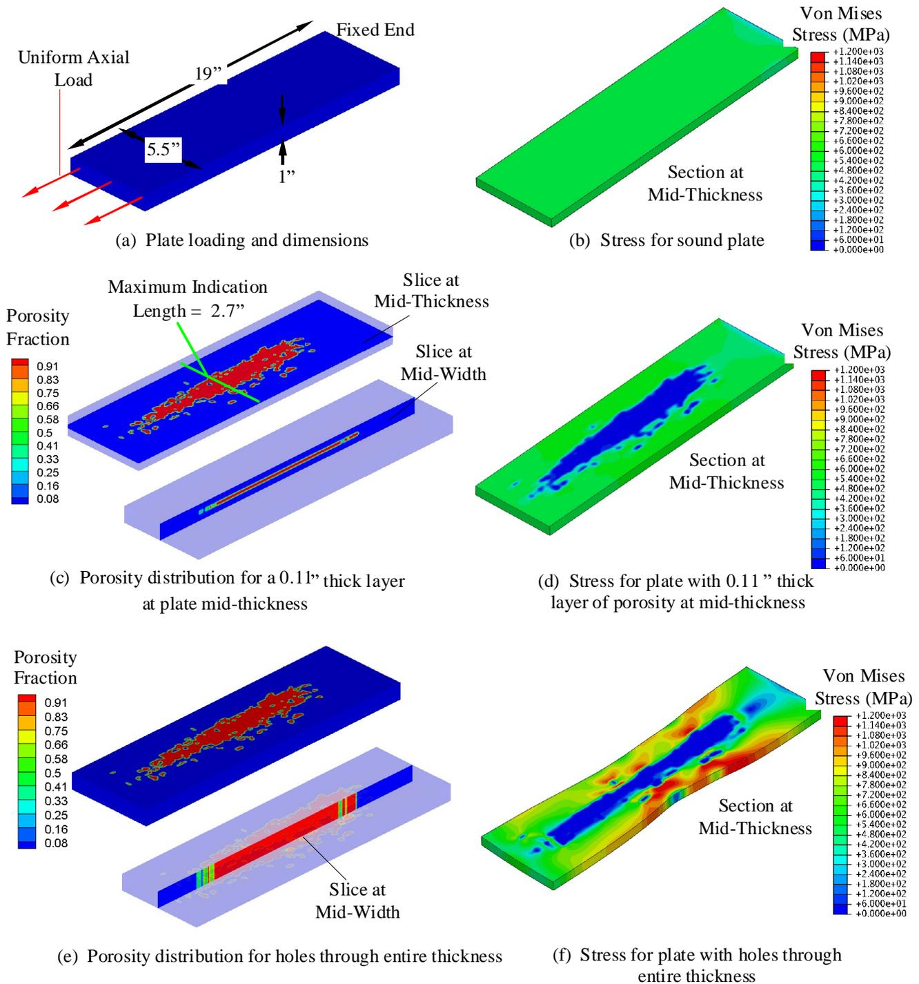
**Fig. 4. Effect of porosity depth on the stresses in an axially loaded plate; the porosity distributions shown in (c) and (e) would give the same indications on a top radiograph.**
