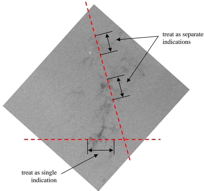
**Fig. 2. Example of the measurement of indication lengths for closely spaced indications.**
