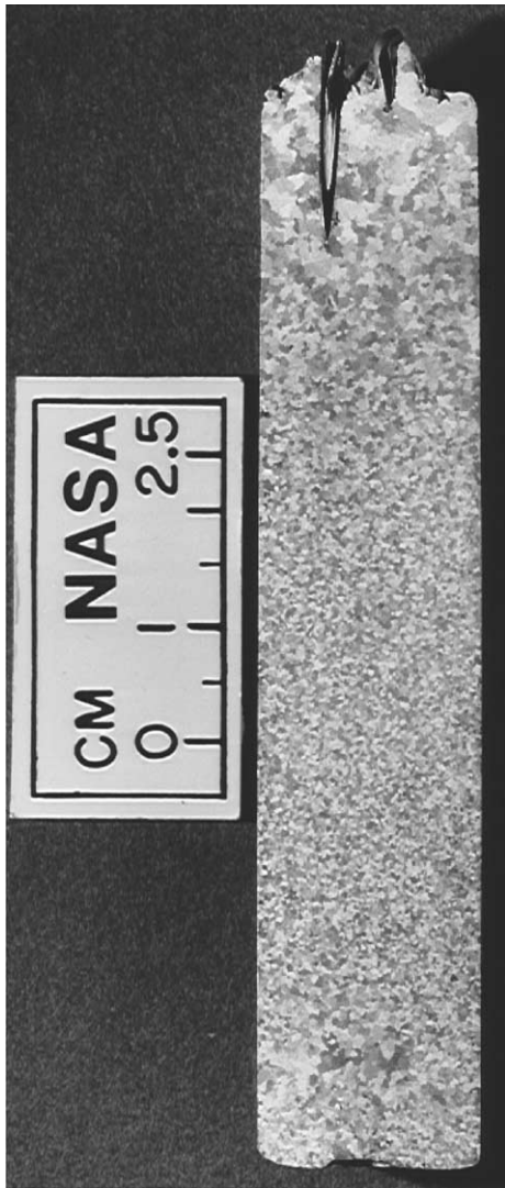
Fig. 5. Longitudinal cross-sectional view of ingot from experiment B10-2, bottom cooled, 16 \text{ K min}^{-1} initial cooling, Al–10wt.%–Cu alloy with 0.045 wt.% \text{TiB}_2
