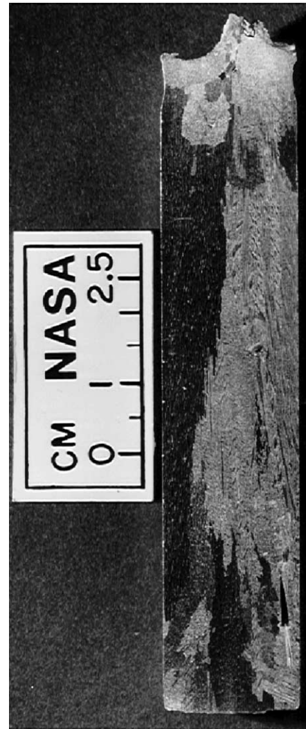
Fig. 6. Ingot from experiment B1-1, bottom cooled, 18.5 \text{ K min}^{-1} initial cooling, Al–1wt.%–Cu with 0.45 wt.% \text{TiB}_2 .
