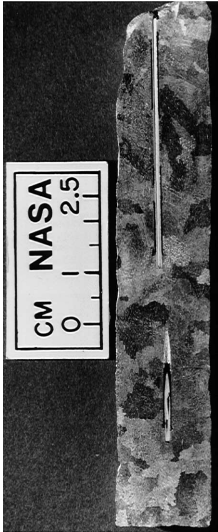
Fig. 9. Experiment T1-1, top cooled, 12 \text{ K min}^{-1} initial cooling, Al-1wt.%-Cu with 0.45 wt.% \text{TiB}_2 .
