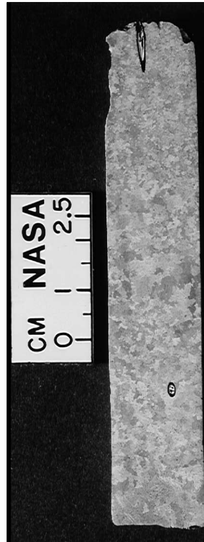
Fig. 8. Experiment T10-2, top cooled, 11.9 \text{ K min}^{-1} initial cooling, Al–10wt.%–Cu with 0.067 wt.% \text{TiB}_2 .
