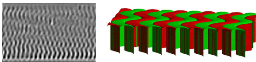
Fig. 7. “Zig-zag” structures in a near-eutectic transparent eutectic alloy \text{CBr}_4\text{--C}_2\text{Cl}_6 . Left: top view of an in situ experiment using an optical long-distance microscope in oblique view and subsequent image processing, G = 100 \text{ K cm}^{-1} , V = 0.5 \mu\text{m s}^{-1} (the growth direction is normal to the plane of the page, the average spacing = 20 \mu\text{m} ) [161]. Right: snapshot of a 3D phase-field simulation of a similar model system [163]. Growth direction is upward.
