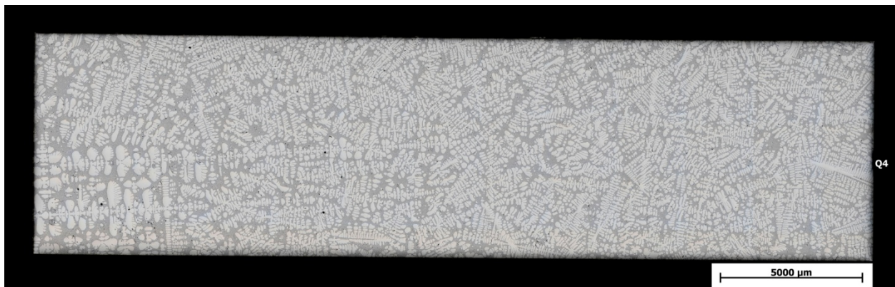
Figure 3: Microstructure in the longitudinal cross-section L4 ( z = 120\text{mm} to 150\text{mm} ) of FM#2 flight sample; direction of solidification from left to right.
