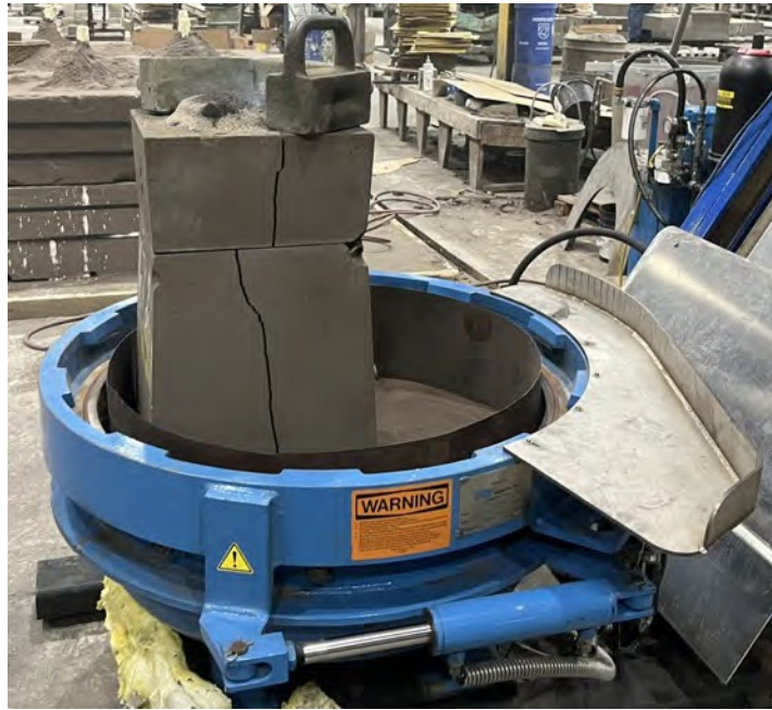
Figure 5: Pressure trial of plate casting at Waukesha Foundry
