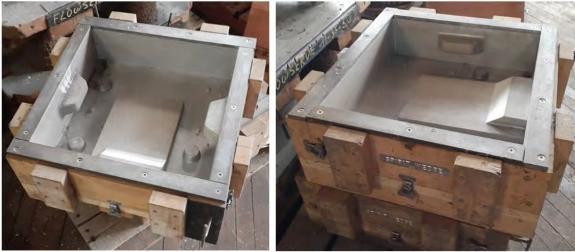
Figure 4: Vertically parted UAB wedge pattern
